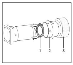
Insert the ring adapter, 1, into the wall pipe.
